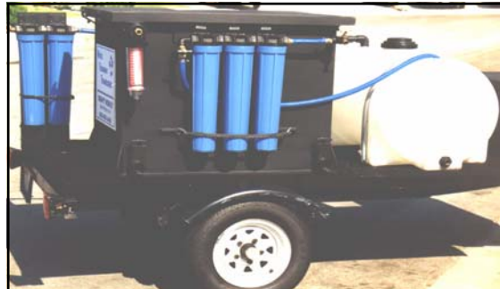
Mobile Water Filtration Units and Water Pickup Devices
