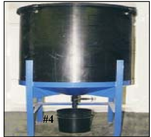
Side view of bottom discharge port
