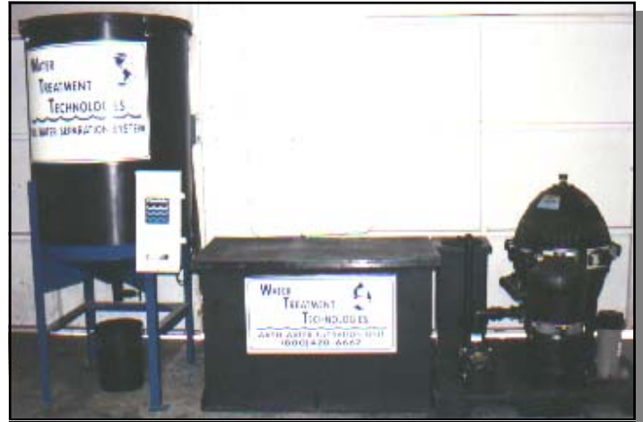
Above ground separator with "ST" water filtration unit, ozone and multi-media polishing system.
